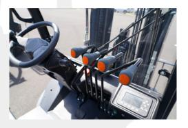
The U-shaped design of the steering wheel and the front-mounted multi-directional valve control make driving easy.
