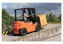
It is equipped with a powerful parking brake, enabling it to park with a load on a 15% gradient in complete safety.
