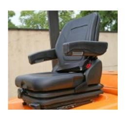
Operator presence system (OPS) - When the operator is not in the driver's seat, the hydraulic controls are activated. The lifting and tilting mechanisms lock automatically and travel is disabled.
