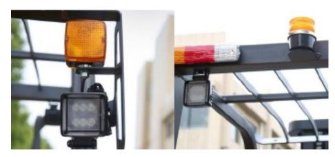
Equipped with LED lamps as standard: rear work lights, headlights, strobe lights and blue LED safety lights. Standard lighting provides optimum visibility and safety.
