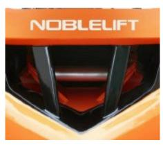
The optimised heat dissipation channel allows a larger radiator to be used, ensuring reliable engine operation even in the most demanding applications.
