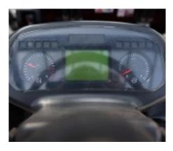
The large LED display and CAN Bus function provide real-time information on the truck's status: parking brake, direction of travel, speed, hour counter, and error codes, fuel level etc...
