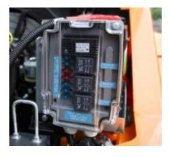
The controller, which incorporates all the electrical components, is protected from temperature, water and vibration by a special, easily accessible casing.
