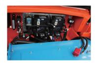
On the FE4P25Q-35Q model, the The drives are positioned high up for efficient ventilation and easy maintenance.
